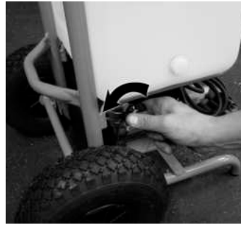
2. Fill tank and open ball valve
