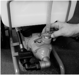
1. Connect pressure hose to pump outlet
